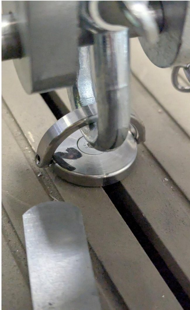
Fixing 1 pullout of 0.35mm at 2.5kN Load
