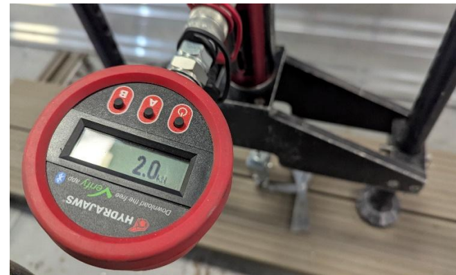
Fixing 2 at 2kN Load
