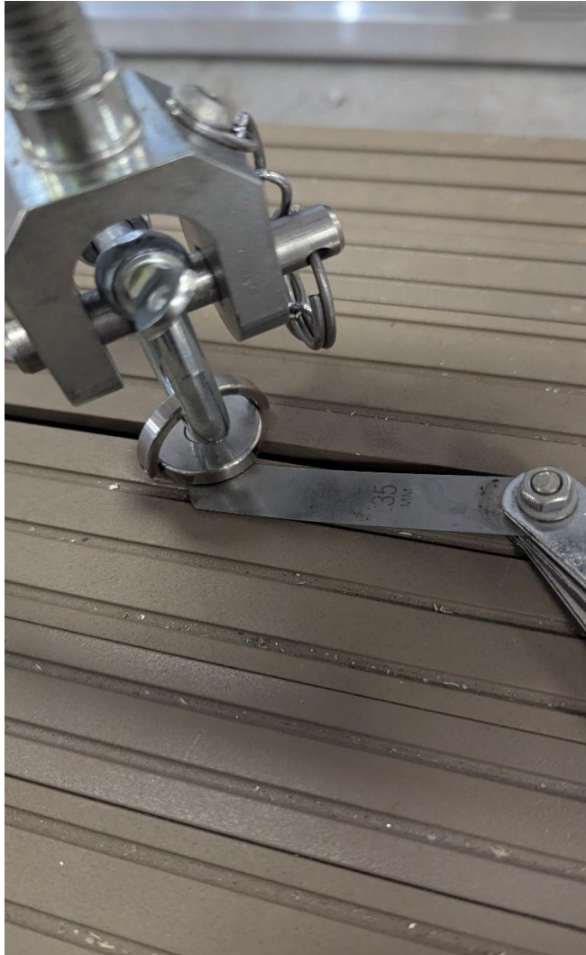
Fixing 1 pullout of 0.35mm at 2kN
