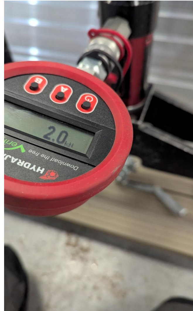
Fixing 1 at 2kN
