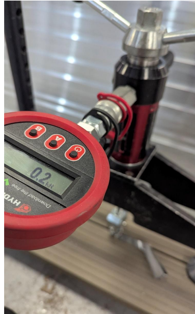
Fixing 2, first movement at 0.2kN
