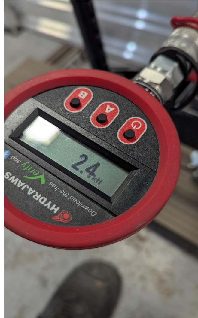
Fixing 1 at 2.4kN Load
