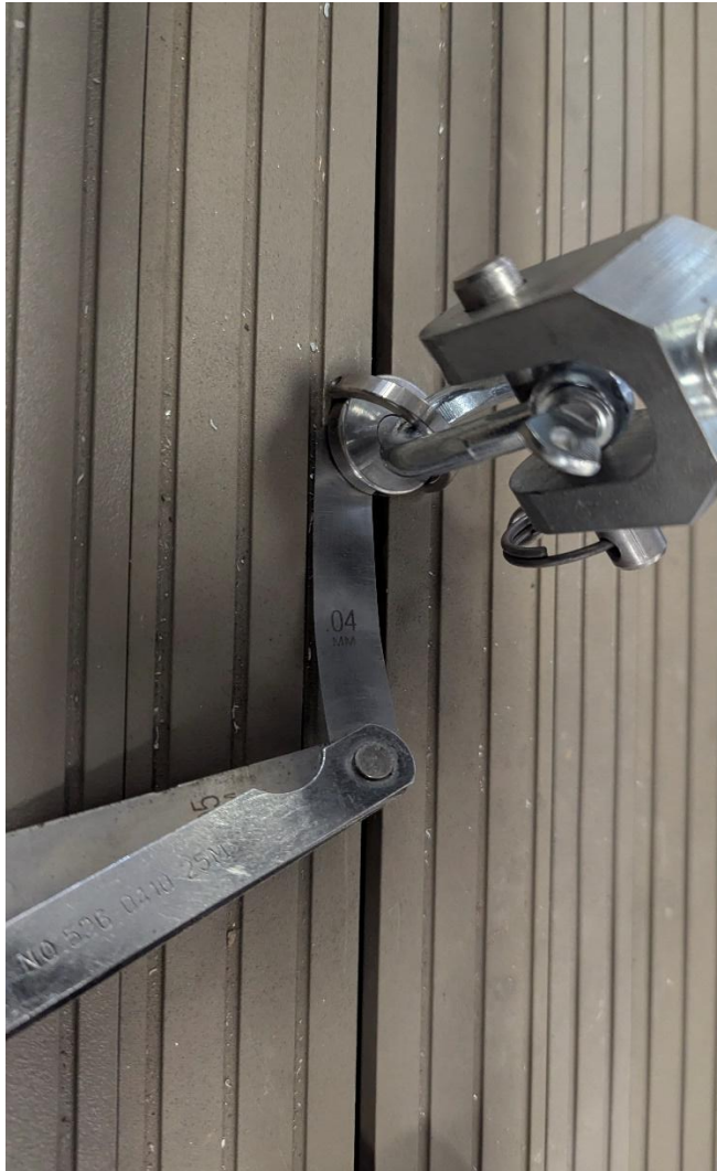
Fixing 1 first movement, 0.04mm
