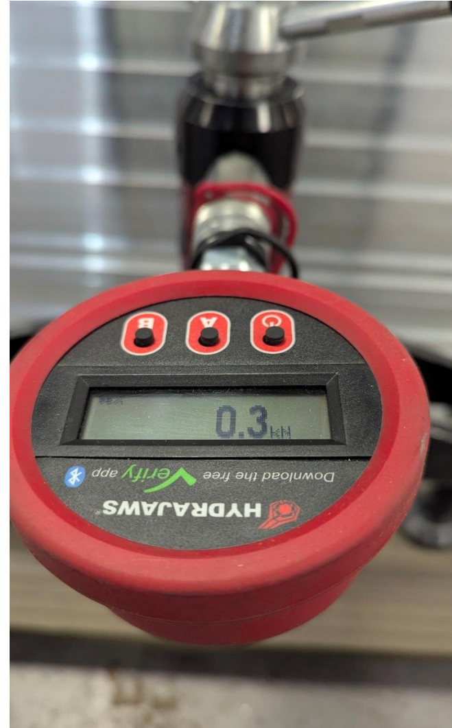
Fixing 1, first movement at 0.3kN
