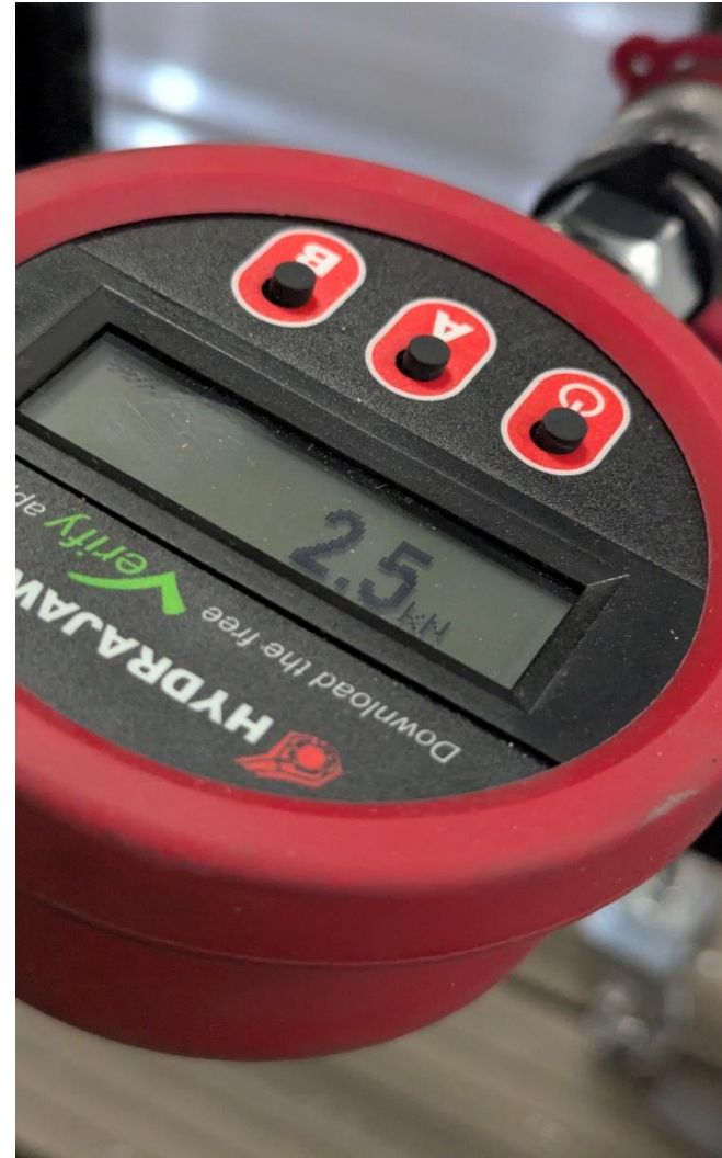
Fixing 2 at 2.5kN Load
