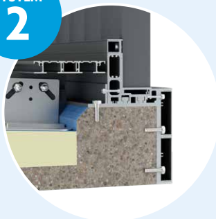
Vertical Infill Balustrade: Concrete Fix 0.74kN Option
