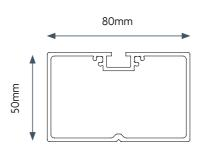
**ECO 50 JOIST SPAN CAPABILITIES:** The Eco 50 Joist can span a maximum of 1000mm between pedestals on a 4kN distributed loading.
