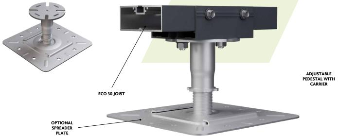
Adjustable Pedestal with carriers are a value engineered product specially designed to offer complete flexibility across an installation with a build-up height minimum of 86mm and maximum 335mm\*. This A fire rated product works seamlessly with all of our joists.
